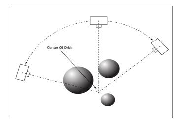
Figure 69 - Rotation around the center of orbit
